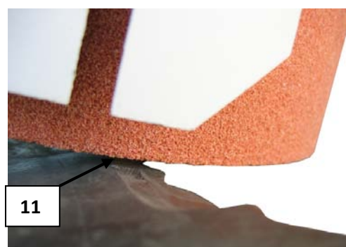
Illustration 6: Grinding angle of knife's edge
