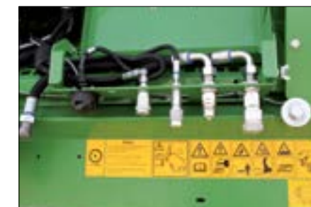
Without use of tools Quick couplings of hydraulic connectors
