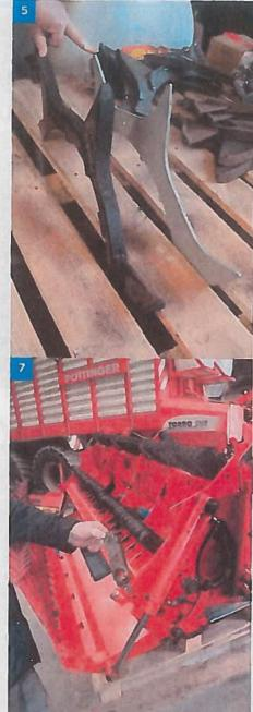
associated moving parts. This is one particularly weak point on Pottinger wagons, which have a greater-thanaverage number of small components prone to wear. Assessing this is tricky without pulling the whole bank out, but swinging it out from under the body will give an indication of its condition.
